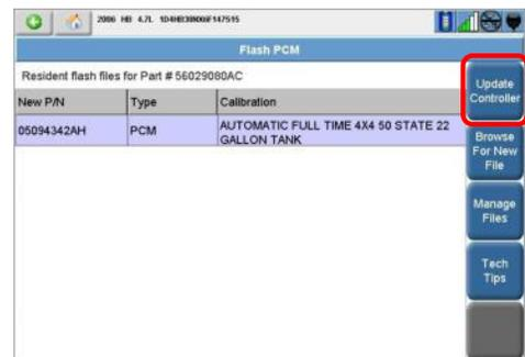
f. Select **OK** when the ECU update is complete and check that the new part number is shown at the top of the screen.
