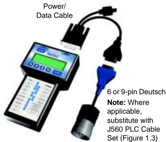
Figure 1.2 Connectivity diagram for ABS diagnostics.
