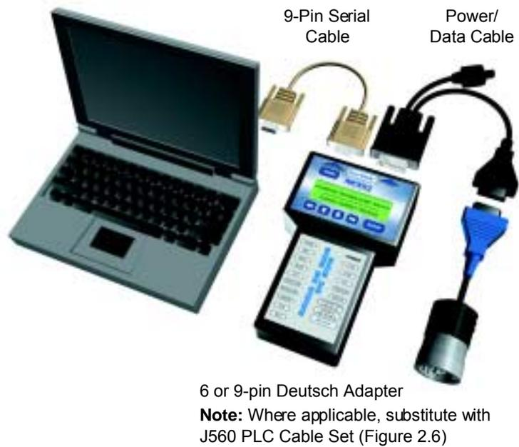
Figure 2.4 Connectivity diagram to Interface the PC with the Vehicle
