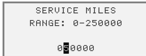
Use the **←** and **→** keys to position the cursor on the digit(s) you wish to edit; then, use the **▲** and **▼** keys to set the value of the digit(s).
