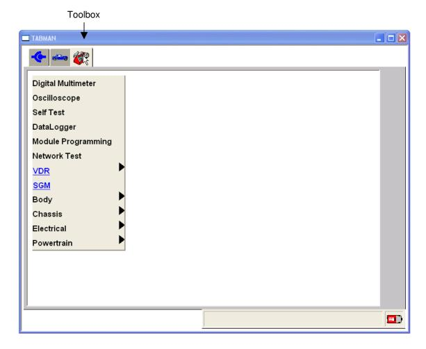
NOTE: Any test can be exited by selecting the menu button on the right side of the screen.
