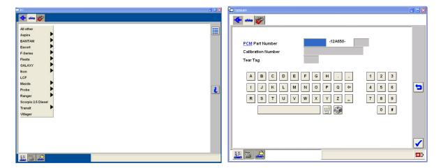
Selecting the tick mark on this screen provides a screen that gives a description of the vehicle. In addition, the Toolbox tab is then populated with the available diagnostics.
