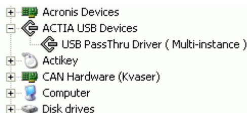
8. When you want to switch back device to normal mode (to be able to work with MultiDiag Office or with generic PassThru software) you should reprogram device back to its original state. Connect device to PC **using RS232 cable (USB cable will not work!!)**, power it on, then run from the desktop *PassThru restore* and follow instructions on screen. You should see this screen:
